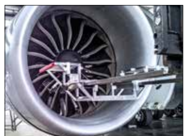
Lifting of the engine podium by forklift
