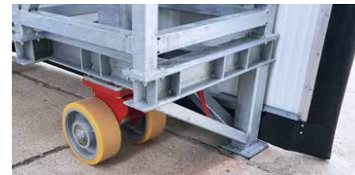
400 mm Castors; Rubber Covers with a height of 40 to 50 cm
